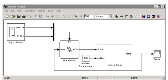
The output signal of the Mux block connects to the input trigger port of the Stateflow block. Your chart should look like this:
