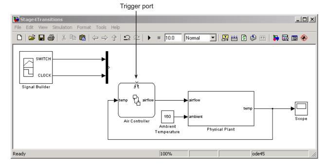
When you define one or more input events for a chart, Stateflow software adds a single trigger port to the block. External Simulink blocks can trigger the input events via a signal or vector of signals connected to the trigger port.
