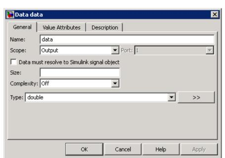
The Data properties dialog box opens on your desktop, this time with different default values, associated with the scope **Output**:
