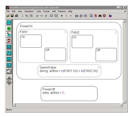
The Boolean expression in (FAN1.0n) is true — and its value equals 1 — if the On state of FAN1 is active. If FAN1 is not on — that is, its Off state is active or power is off — then in (FAN1.0n) equals 0. Similarly, the value of in(FAN2.0n) represents whether FAN2 is on or off. Therefore, the sum of these Boolean expressions indicates whether 0, 1, or 2 fans are operating during each time step.
