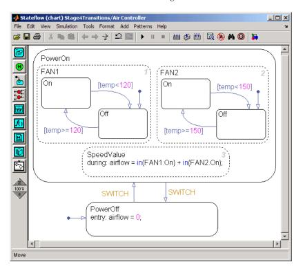
Now that you have associated these transitions with the event SWITCH, the control system will alternately power on and off every time SWITCH occurs — that is, every time the chart detects a rising or falling signal edge.
