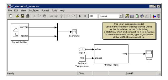
The model is incomplete because it does not include the Stateflow chart that you will build as you work through the exercises in this guide. Instead, the model contains several nonfunctional blocks: the Terminator, Inport, and Annotation blocks, as shown:
